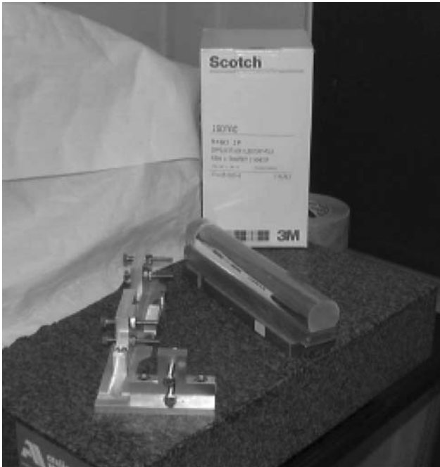
Figure 25.14 Fixation with a special jig of a crystal on a processing reference base.
