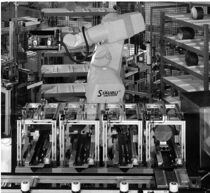
Figure 24.18 Fully automatic measuring and mounting ingot station using a robot-driven handling tool.
