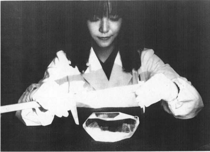
Figure 20.6 Photograph of LAP crystal with dimensions of 7 \times 8 \times 18 \text{ cm}^3 .
