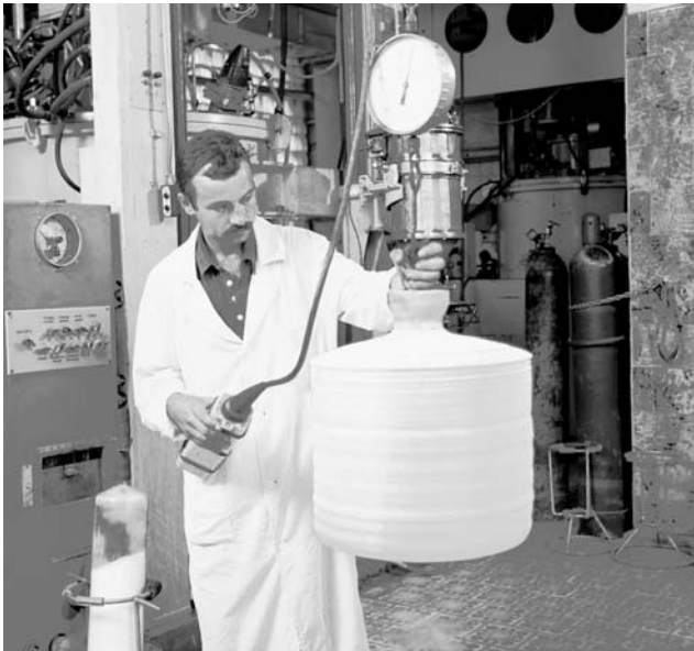
Figure 23.6 Typical CsI(Tl) crystal, grown in the 'Crystal-500' installation: seed diameter – 70 mm; crystal diameter – 450 mm.
