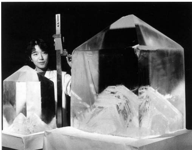
Figure 20.1 KDP crystals (size 45 \times 45 \times 70 \text{ cm}^3 , growth period one year).
