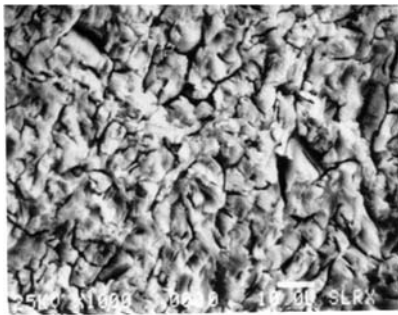
ID Depth of damage : 30 \mu\text{m} Magnification 1000 \times
