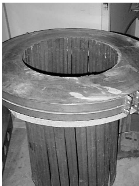
Figure 21.4 Photograph of the cold container of 'Crystal-405' skull-melting furnace.
