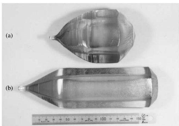
Figure 19.6 \text{La}_3\text{Ta}_{0.5}\text{Ga}_{5.5}\text{O}_{14} single crystals of (a) 3 and (b) 2 inch diameter.
