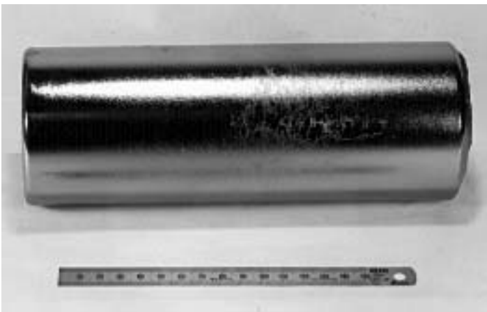
Figure 15.10 75-mm diameter undoped GaAs single crystal of 200-mm length.
